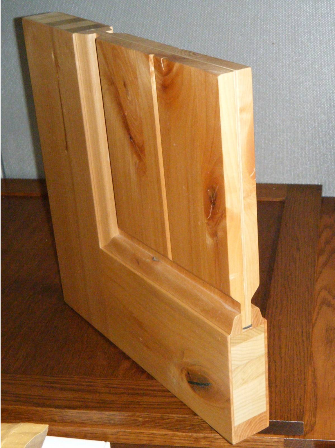
Photo 1 shows a sample of the construction of a wooden panel door commonly used in residential and business occupancies. This type of door cannot meet the test for fire rating under NFPA 252 because of the thin cross-sections of its panels where they join the rails and stiles. A modern door such as this one will be made up of many pieces of
