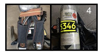
Pull the SCBA out of the bracket, look over all the straps for tears, wear and abrasions, if noted remove from service and send for repairs, ensure the bottle is snug in the harness
