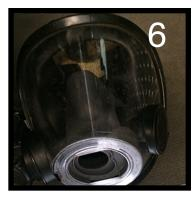
Finally look over your mask, make sure it has no cracks, has a good seal and webbing is not worn
