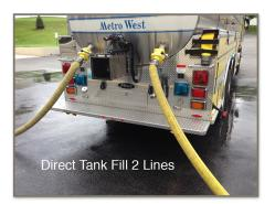
Many tankers/tender have direct fill valves, these allow for open flow of water directly into the tank providing optimal efficiency in filling the apparatus
