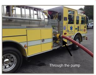
Filling a tanker/tender through the pump is often the least efficient means to quickly fill and return a tanker/tender to the fire ground
