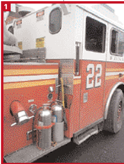
(1) This truck company has two water extinguishers, one with plain water and one with AFFF foam/water, and a set of forcible entry tools right next to the crew cab so the tools can be grabbed quickly. (Photos by author.)
